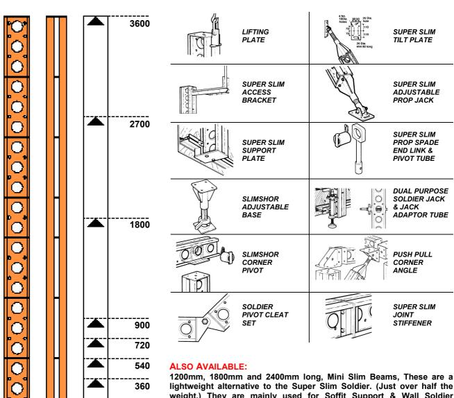
1200mm, 1800mm and 2400mm long, Mini Slim Beams, These are a lightweight alternative to the Super Slim Soldier. (Just over half the weight.) They are mainly used for Soffit Support & Wall Soldier applications. Mini-Slim Beams are compatible with Super Slim Access Brackets and Super Slim Lifting Plates.
